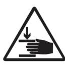
Crushing hazard, e.g. when closing the bed base!
