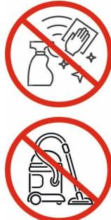
SPECTRA LED boards are very sensitive optical components.
