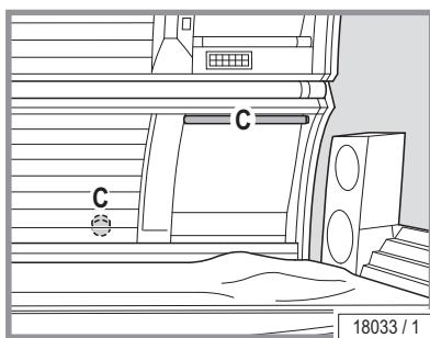
The facial tanner's low pressure lamp must be removed first so that the high pressure lamp can be changed.
