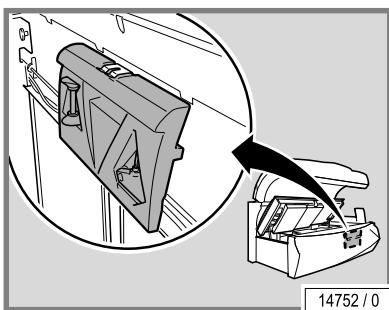
The service kit is fitted on the inside of the front panel.
