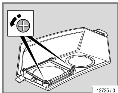
Each of the high pressure lamps in the shoulder tanner is fitted with 2 different filter panels. The two filter panels are secured in place inside the housing.
