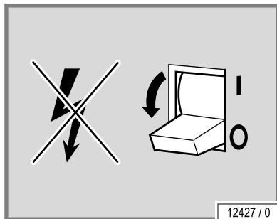
If work is to be performed on the devices, they must be deenergized. That means that all live cables must be switched off.
