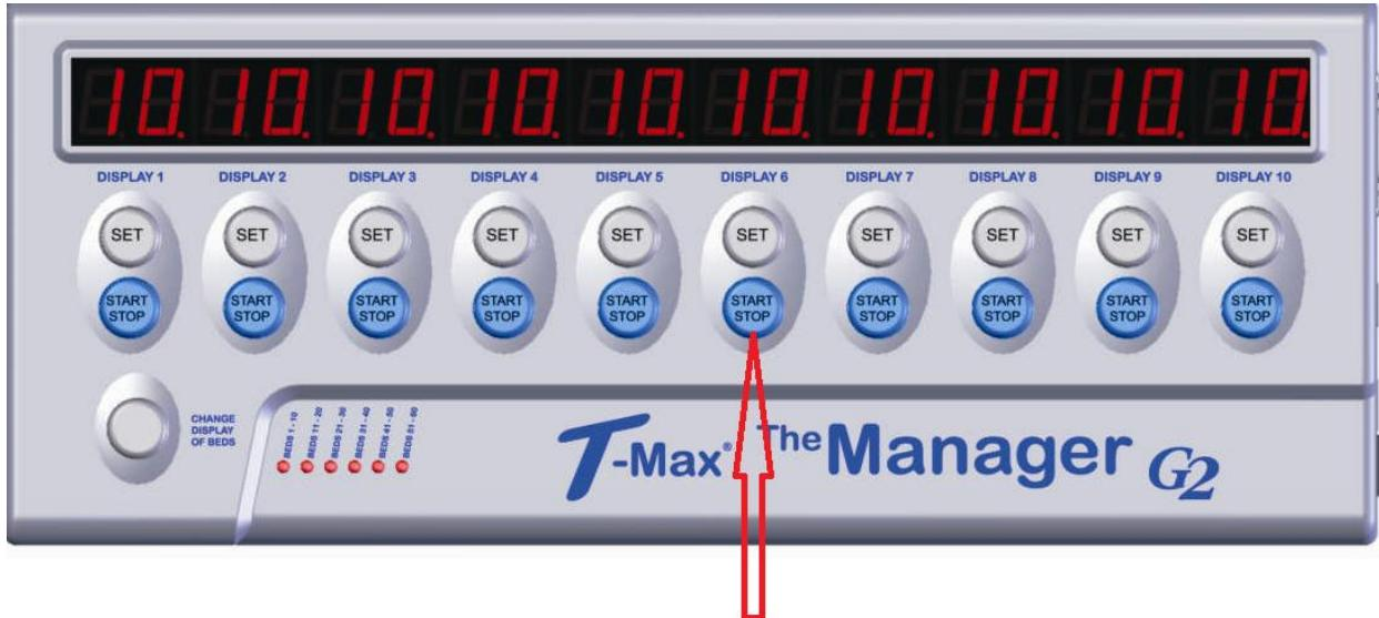
9. Press the START/STOP button Display 6 and the lamp hours will now show in Display 7 and Display 8.
