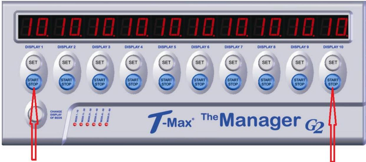
2. Press the Start/Stop Button under displays 1 and 10 on the T-Max® Mgr G2 at the same time until the displays change and show zeros in displays 6, 7 and 8. Release the Start/Stop Buttons.
