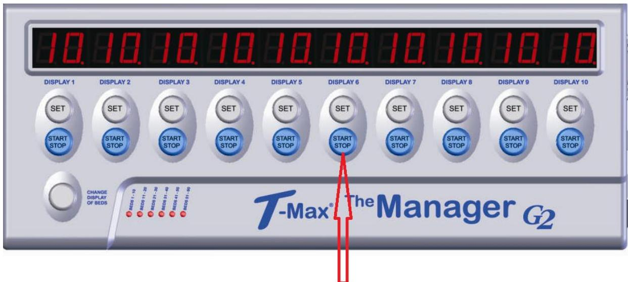
8. Set Display 6 with the SET button to a value of 6 for lamp hours.
