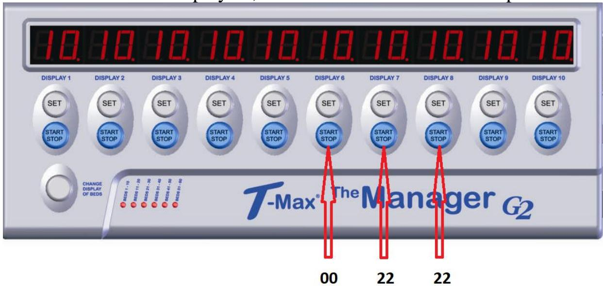
3. Press the Set buttons under displays 6, 7 and 8 until the number for security level 2 is displayed.
