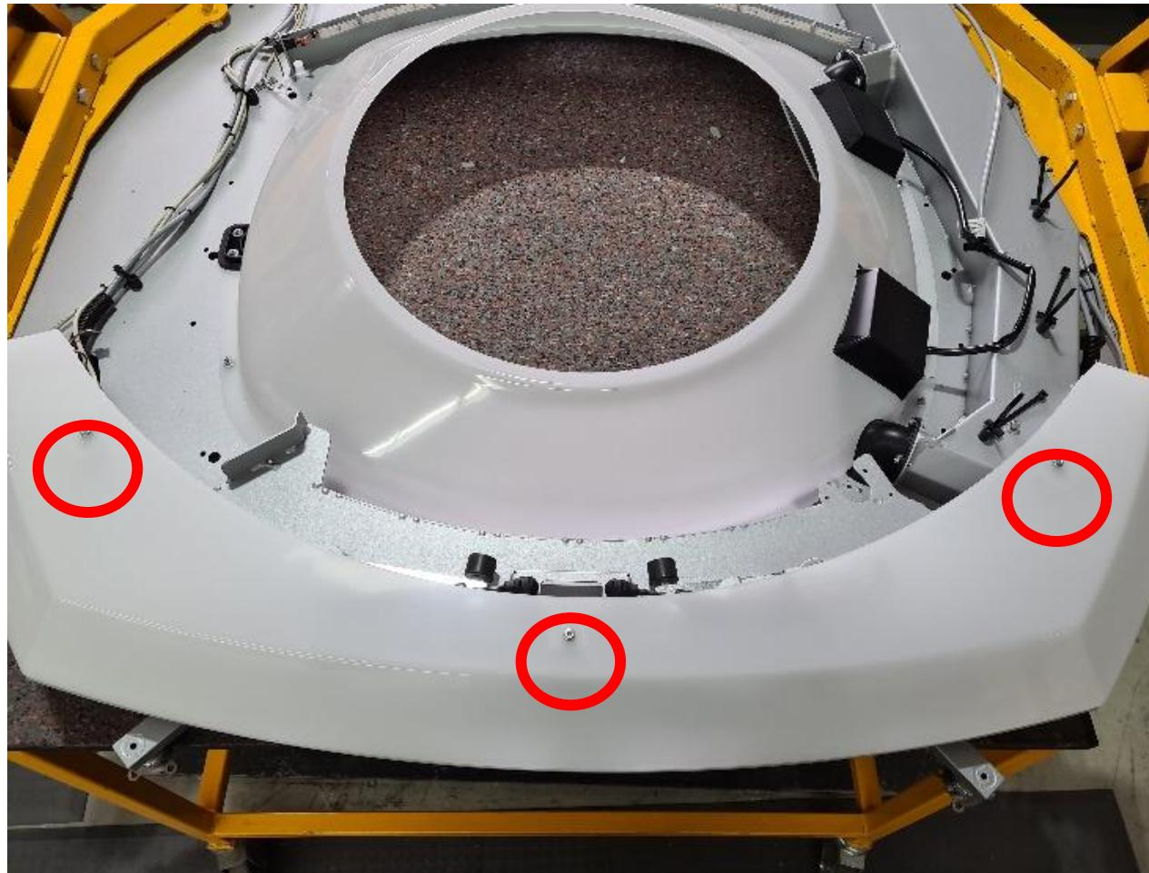
It has (3) T-25 screws fastening it to the roof, if you need to remove it to access the shocks.
