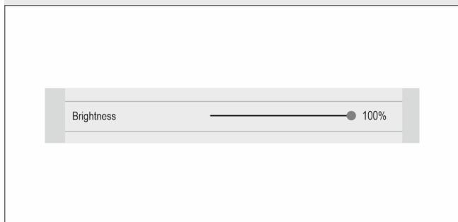
By moving the slider, you can change the brightness of the LED lighting (20%, 40%, 60%, 80% and 100%).
